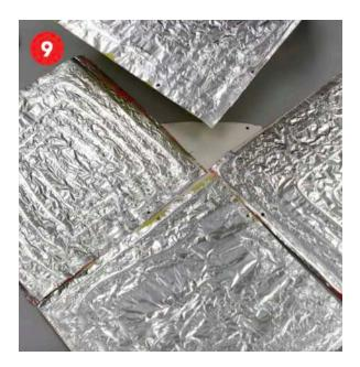
To assemble the solar cooker, place the four larger squares on top of the unfoiled small square.
